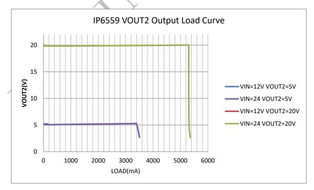
Figure 5. IP6559 VOUT2 output load curve
