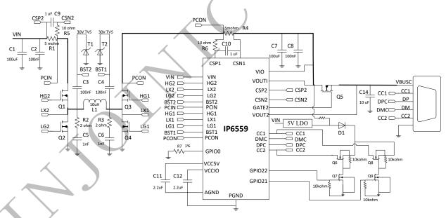
Figure 9. Typical application schematic diagram of IP6559 single C port with EMARK identification output
