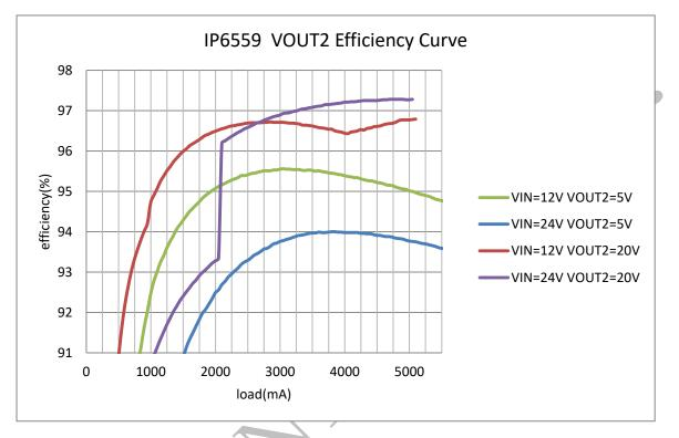
Figure 4. IP6559 VOS1 output efficiency curve
