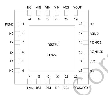
Fig. 3 IP6537U PIN Configuration
