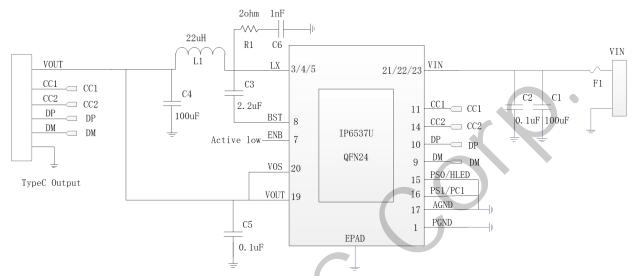
Fig. 7 IP6537U Application Schematic of Single Type-C Port PD Fast Charging Output
