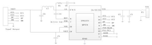
Fig.1 IP6537U Simplified Application Schematic
