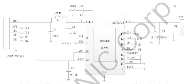
Fig. 2 IP6537U Application Schematic of Single Type-C Port PD Fast Charging Output
