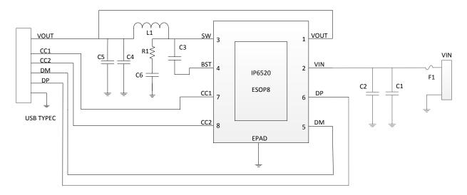
Figure 1 IP6520 simplified application schematic
