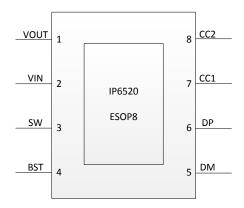
Figure 2 Pin Assignment
