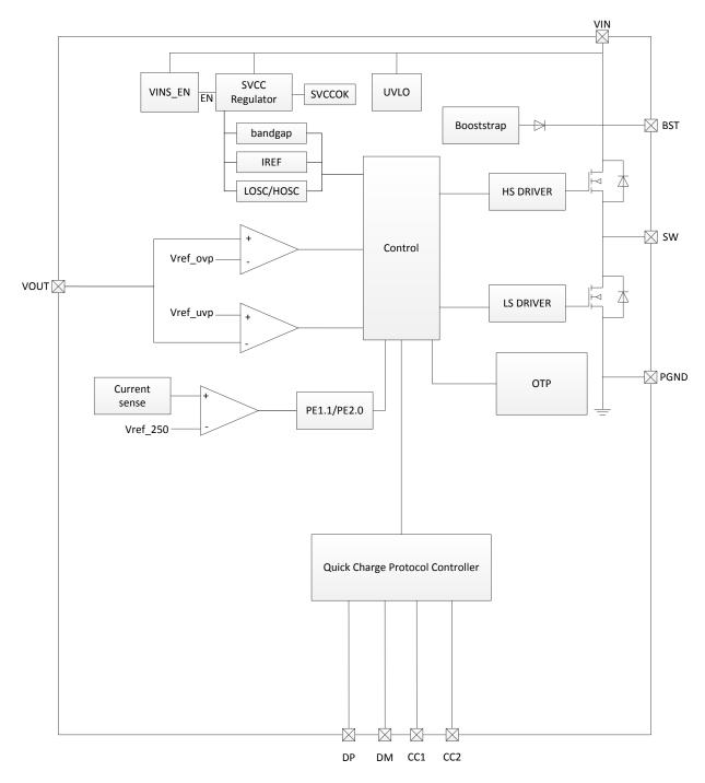
Figure 3 IP6520 Internal block diagram
