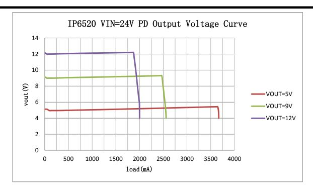
Figure 5 IP6520 VIN=24V PD output VOUT-IOUT curve
