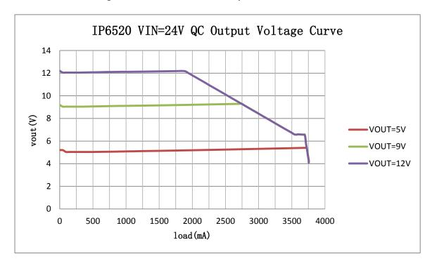
Figure 6 IP6520 VIN=24V QC output VOUT-IOUT curve
