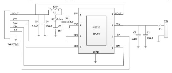
Figure 7 Type-C port PD fast charge output application schematic
