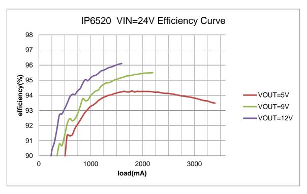
Figure4 IP6520 VIN=24V Efficiency Curve
