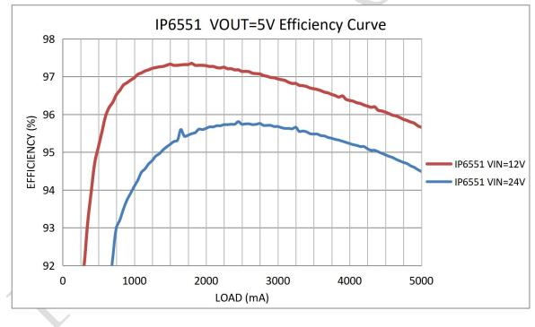
Figure 6.IP6551 VOUT=5V output efficiency curve
