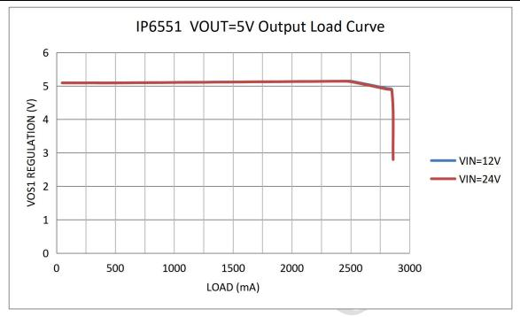
Figure 7.IP6551 VOUT-IOUT curve
