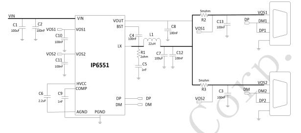
Figure 2. IP6551 dual USB A output ports application schematic diagram
