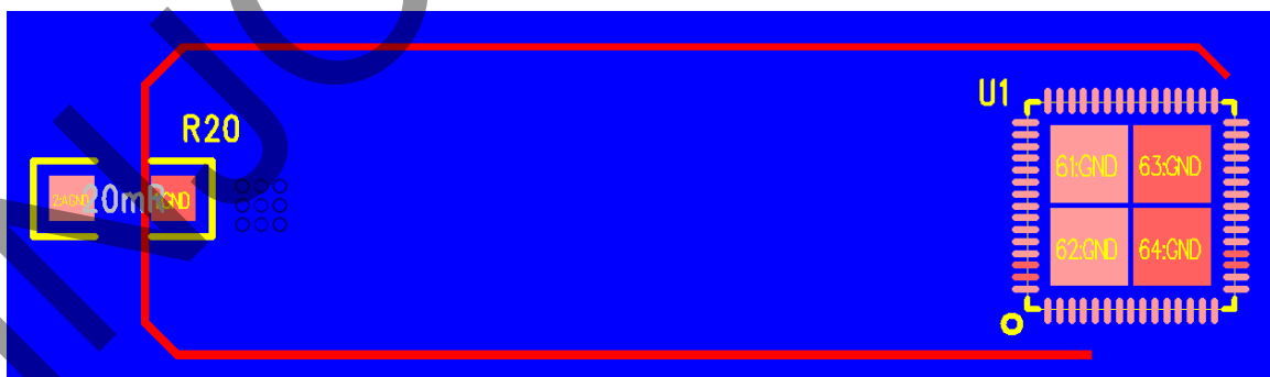
Figure31 Wireless charging sampling resistance wiring
